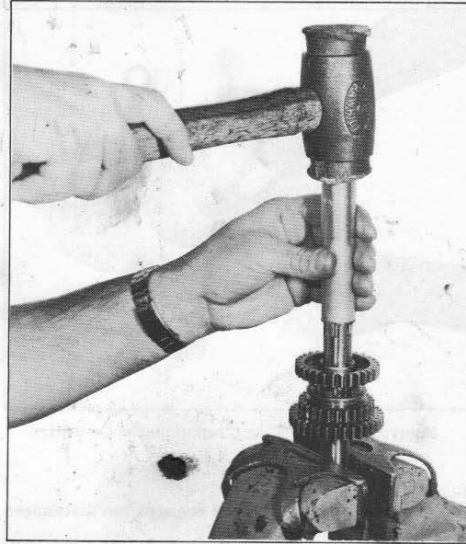
Figure 4.14. Assembling Gear Snap Ring on Shaft
