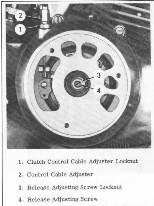
Figure 4.7. Clutch Adjustments
