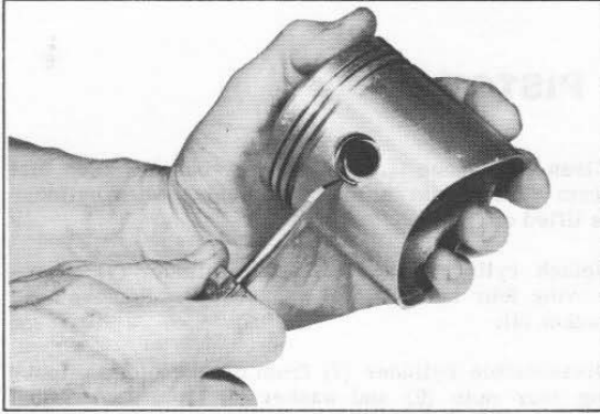
Figure 3.5. Removing Pin Retaining Ring
