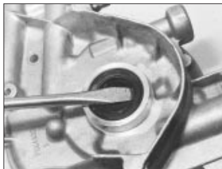
5B.77A Removing the oil pump seal
