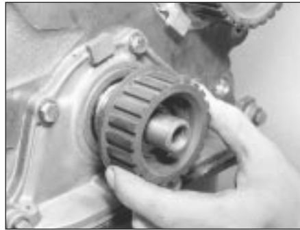
42.20 Fitting crankshaft timing belt sprocket
