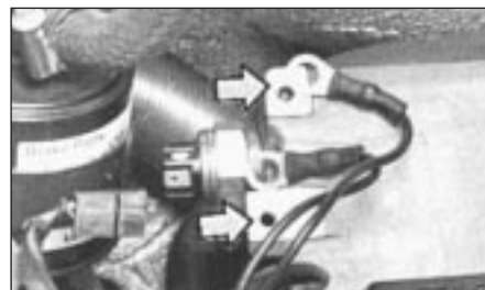
Fig. 13.59 Disconnecting the earth leads (arrowed) on the 1372 cc Turbo ie engine (Sec 9E)
