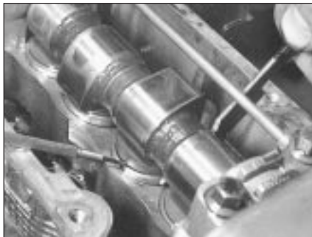
5B.1B Using a modified C-spanner and screwdriver to remove a shim
