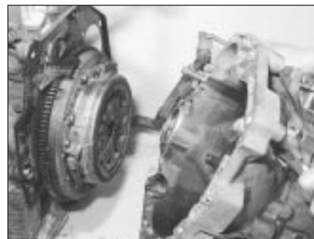
5C.39 Separating the engine and transmission
