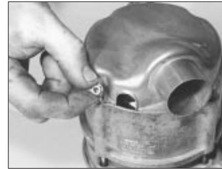
15.12B Alternator rear cover and fixing nut
