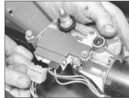
15.98C . . . and detach the wiring connector
