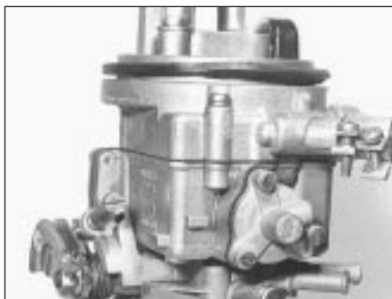
9B.2A Weber 32 TLF 4/250 carburettor from anti-run-on solenoid valve side
