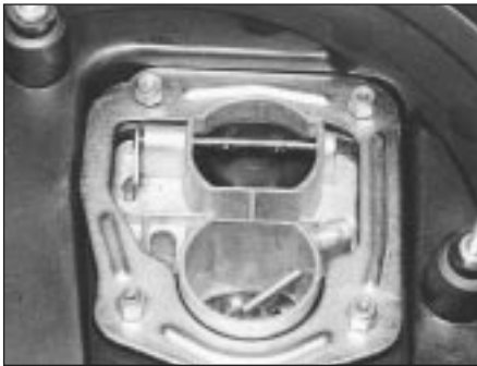
9A.9A Circular type air cleaner fixing nuts
