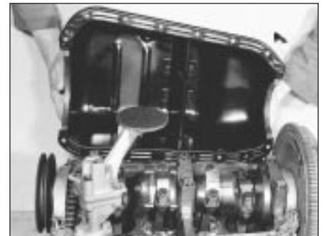
8.7A Fitting the sump pan
