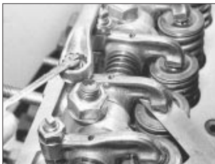
5.7 Adjusting a valve clearance
