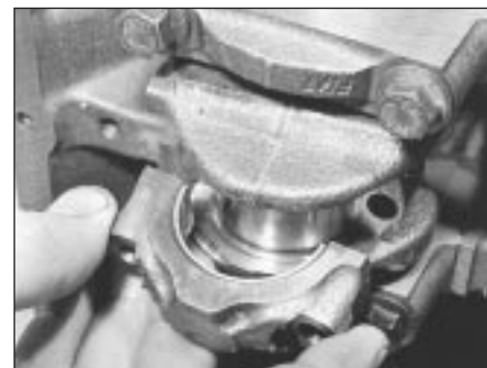
5B.98 Fitting a big-end bearing cap
