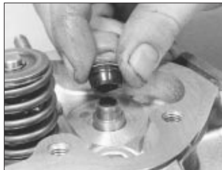
39.7 Valve stem oil seal
