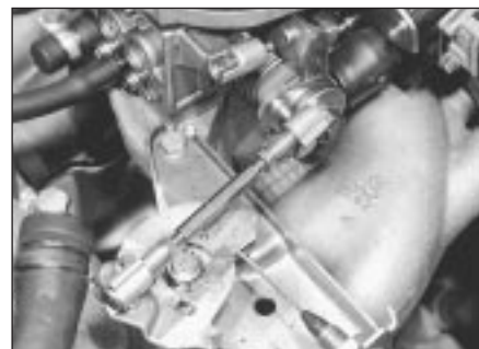
9D.22 Accelerator control rod and cable connections
