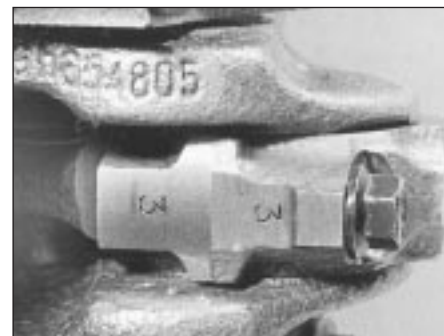
5B.88 Connecting rod and cap numbers
