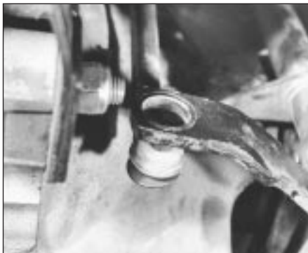
5C.24B Gearchange rod with ball socket connection
