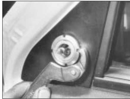
24.3 Mirror ring nut and C-spanner
