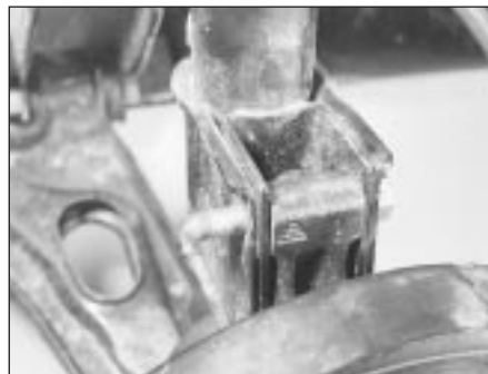
3.3 Strut clamp bolt
