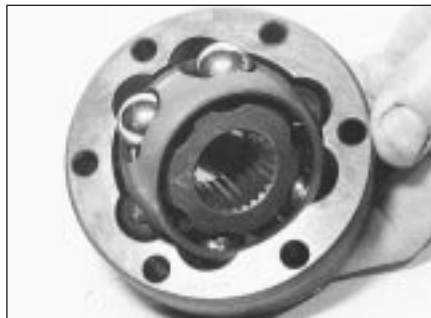
13.18 Removing inboard CV joint ball/cage assembly from outer track
