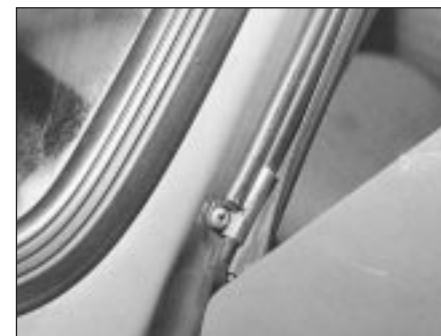
15.108B Pillar lower screw for aerial
