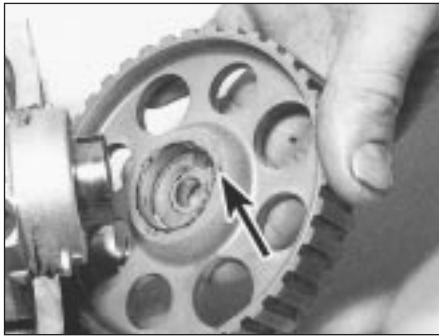
5B.22C Camshaft sprocket showing integral key (arrowed)
