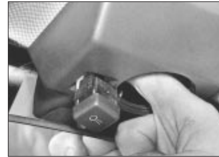
15.81 Roof-mounted spotlamp switch removal
