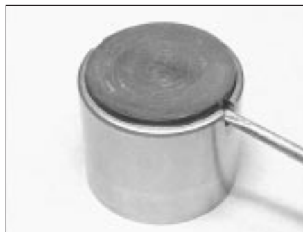
26.2 Removing a shim from a cam follower
