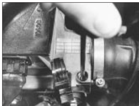
9C.36 Using an Allen key to adjust the mixture (CO level)
