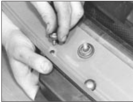
15.98A Remove the wiper motor retaining screws . . .
