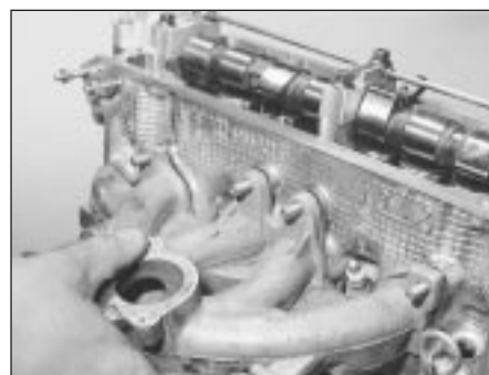
5D.25B Fitting the inlet manifold
