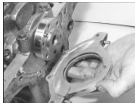
5D.9 Fitting crankshaft rear oil seal retainer
