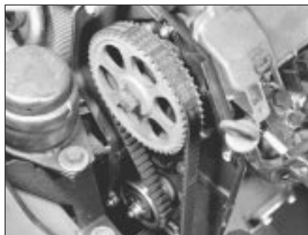
7B.52A Timing belt refitted over the sprockets and tensioner
