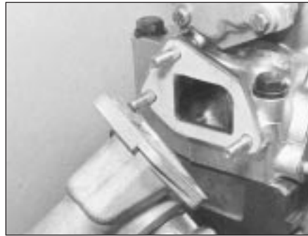
4.4 Fitting thermostat housing (1116 cc engine)
