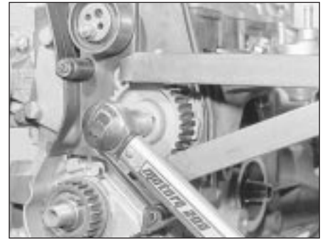
7B.46 Tightening the auxiliary shaft sprocket bolt
