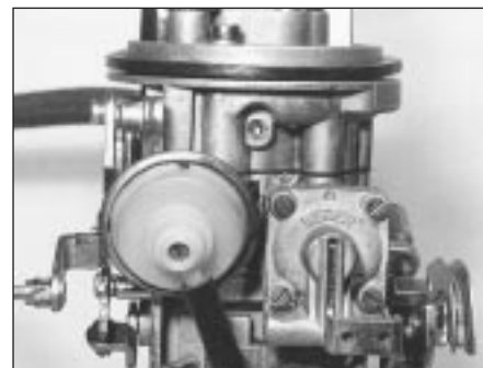
9B.2C Weber 32 TLF 4/250 carburettor from accelerator pump side
