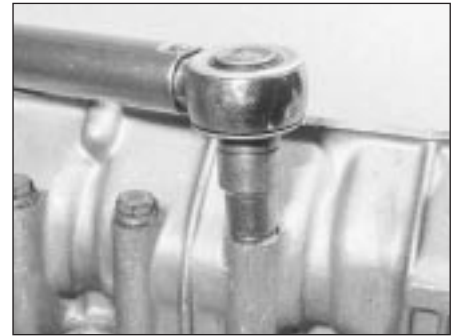
27.18 Tightening a camshaft carrier bolt
