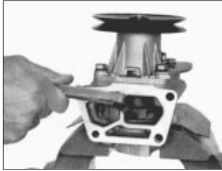
Fig. 2.6 Checking impeller clearance (Sec 9)
