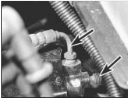
11.25 Clutch operating cylinder showing hydraulic line connection and bleed nipple (arrowed)
