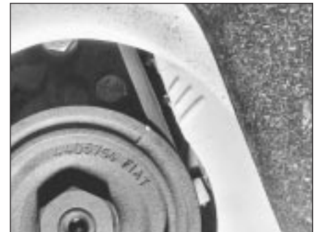
4.4 Ignition timing marks on belt cover
