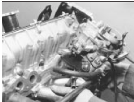
19.4C Fitting intake manifold complete with carburettor
