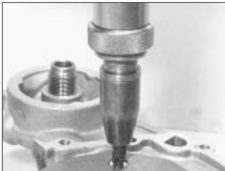
5B.73 Removing the oil pump rear cover plate screws
