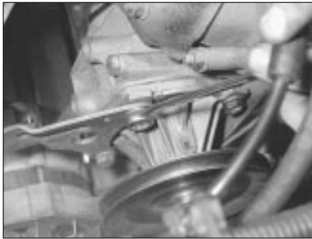
8C.40 Coolant pump/alternator bracket bolt removal
