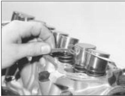
7B.82 Locating a new camshaft housing gasket on the cylinder head
