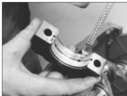
7D.9 . . . and lubricate the shells
