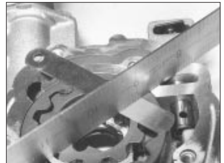
5B.74B Checking the oil pump gear endfloat
