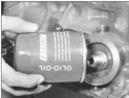
2.8 Screwing on the oil filter (903 cc)
