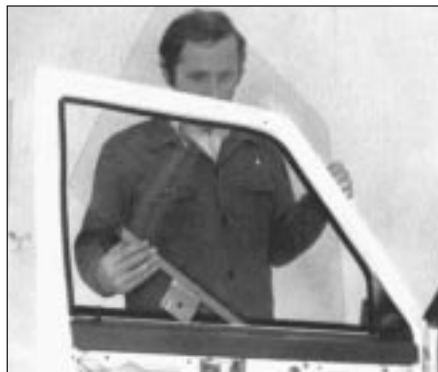
Fig. 12.8 Removing door glass (Sec 12)
