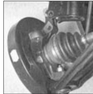
Fig. 1.18 Hub carrier detached from strut clamp (Sec 13)
