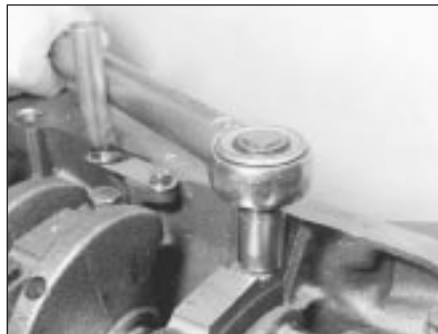
42.4B Tightening a main bearing cap bolt
