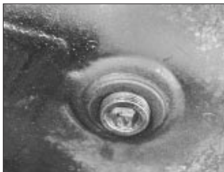
7A.12A Engine sump drain plug - 1372 cc engine
