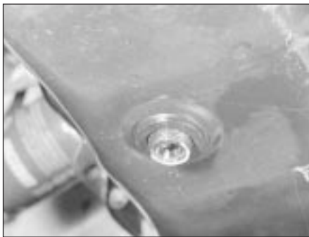
2.6 Engine sump drain plug
