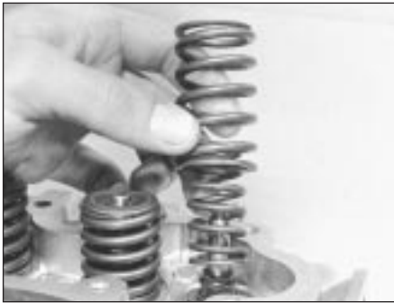
39.4B Double valve springs
