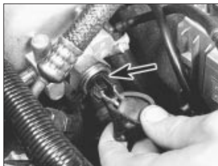
9F.5 Maximum air pressure switch (arrowed)
