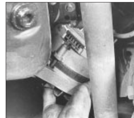
15.4 Removing the alternator from the 999 cc engine
