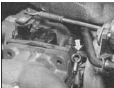
Fig. 13.64 Turbocharger oil supply pipe connection (arrowed) (Sec 9F)
