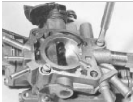
9B.26D Extracting the throttle valve block screws from the Weber 32 TLF carburettor
