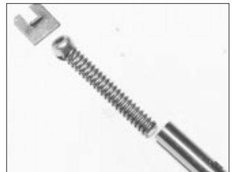
5B.72B Oil pump relief valve components
