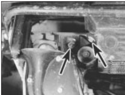
6B.25 Oil cooler mounting bolts (arrowed)
