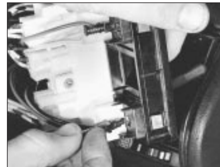
15.54B Disconnecting a fibre optic cable from its holder on the 1301 cc Turbo ie model
