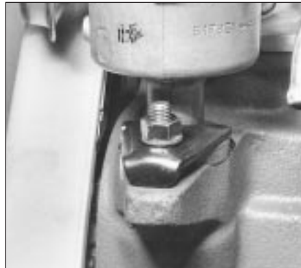
4.5 Distributor clamp plate nut
