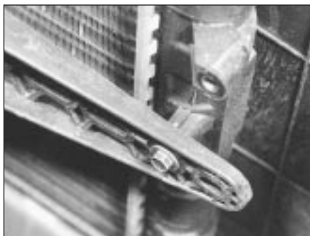
8C.22 Cooling fan to radiator securing bolt
