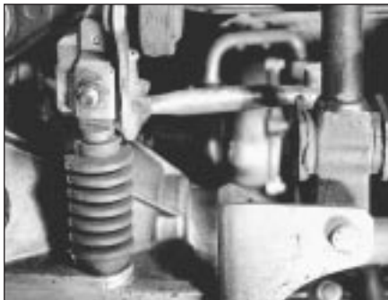
12A.5 Gearchange rod connections at transmission (1301 cc Turbo ie engine)
