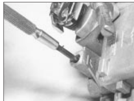
9B.9 Mixture adjustment - Weber 32 TLF carburettor
