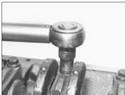
5D.7A Initial tightening of a main bearing cap bolt
