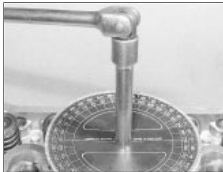
29.24 Tightening a cylinder head bolt through 90° using a protractor
