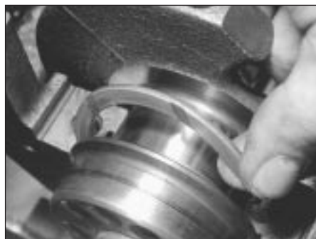
7D.7A Locate the thrust washer . . .
