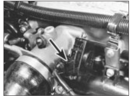
9C.90 Throttle position switch (wiring plug arrowed)
