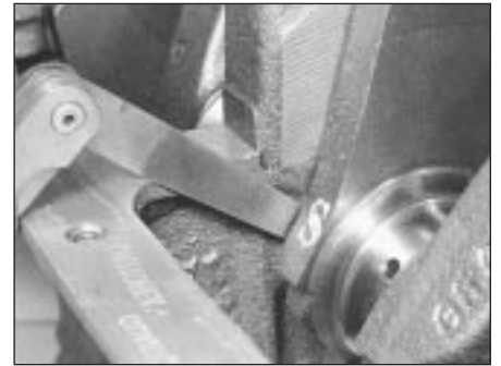
20.10 Checking crankshaft end float
