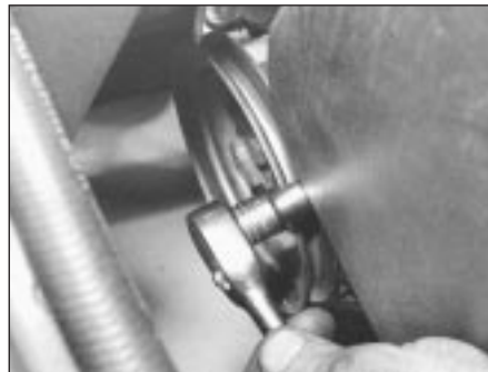
5B.6 Timing cover lower fixing bolt removal
