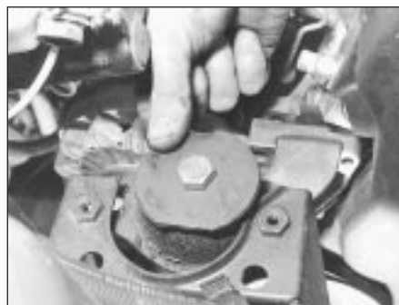
5C.31A Right-hand engine mounting disconnected
