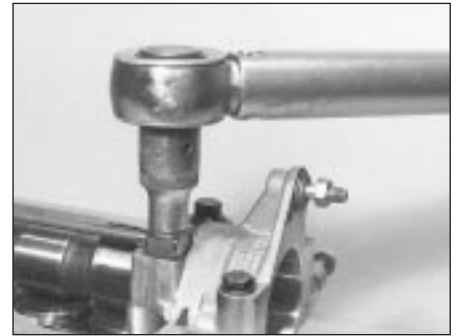
5B.23B Unscrewing the camshaft bearing/banjo union bolt
