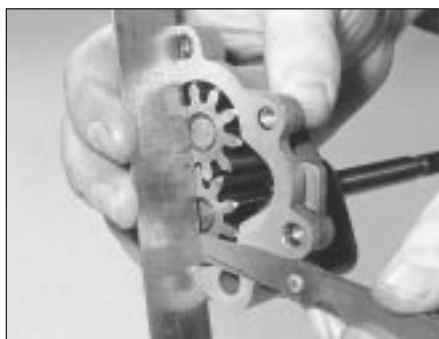
7B.177 Checking the gear endfloat
