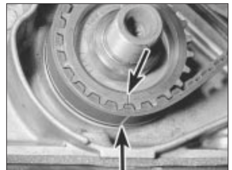
7B.52B Timing belt mark aligned with scribed mark on crankshaft sprocket (arrowed)
