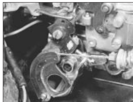
9B.37B Throttle cable connection on the Weber 30/32 DMTE carburettor
