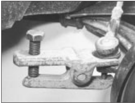
2.2 Disconnecting a tie-rod end balljoint
