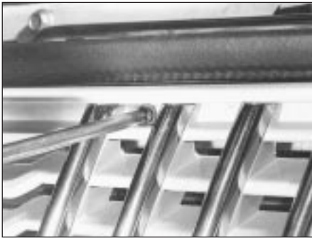
17.19A Extracting a radiator grille screw
