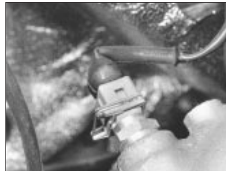
7C.18 Engine coolant temperature sender and wiring connector
