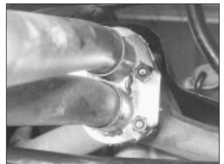
44.15 Exhaust downpipe flange nuts
