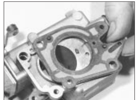
9B.26E Throttle valve block gasket on the Weber 32 TLF carburettor
