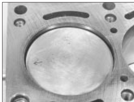
5B.96 Piston directional arrow
