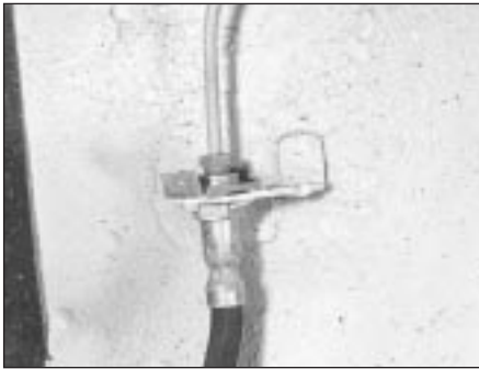
11.3 Front hydraulic hose bracket
