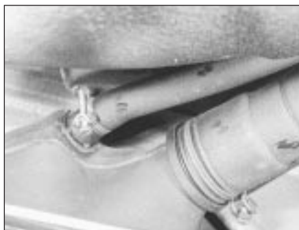
5.3 Fuel tank filler and vent hoses
