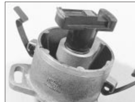
10.41A Distributor body showing elongated slots in the mounting lugs
