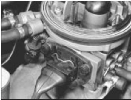
7C.20 Fuel injector wiring connection
