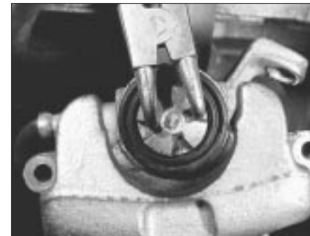
14B.28 Rotating a rear caliper piston
