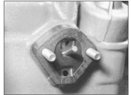
3.6B Fuel pump spacer and pushrod
