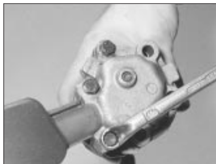
7B.171 Undo the oil pump cover bolts
