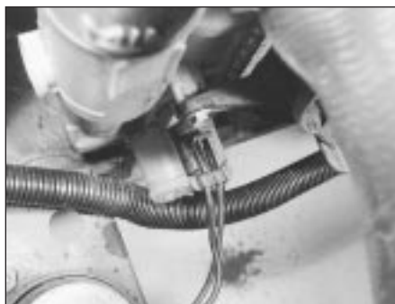
5C.19C Radiator fan cut-out thermostatic switch
