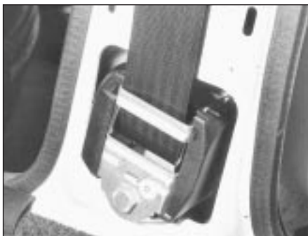
23.3 Front seat belt lower mounting
