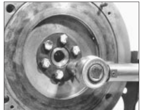
20.14 Tightening flywheel bolts
