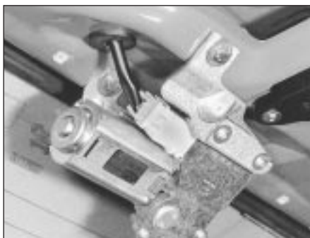
15.106 Tailgate wiper motor - later model
