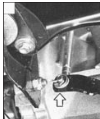
Fig. 13.24 Disconnect the gear selector rod at the connection indicated on the 1372 cc ie and Turbo ie engines (Sec 7C)
