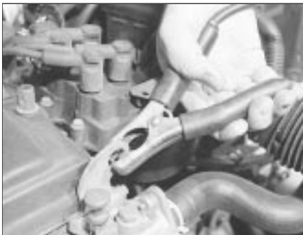
4 Connect the other end of the black jump lead to a bolt or bracket on the engine block, well away from the battery, on the vehicle to be started.
