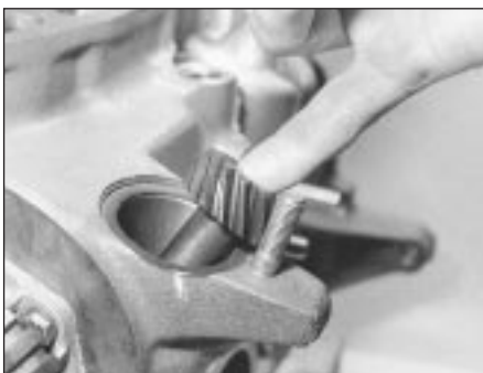
42.15 Fitting oil pump driveshaft
