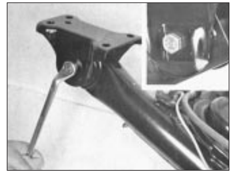
Fig. 11.9 Removing trailing arm pivot bolt (Sec 10)
