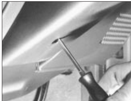
15.45A Undo the retaining screws . . .
