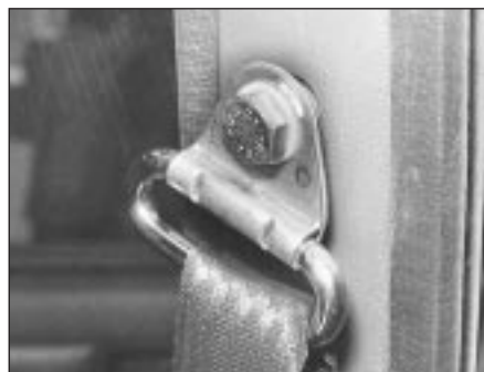
23.5 Front seat belt upper mounting
