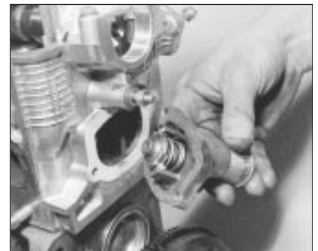
8A.9 Fitting the thermostat housing. Note the new gasket
