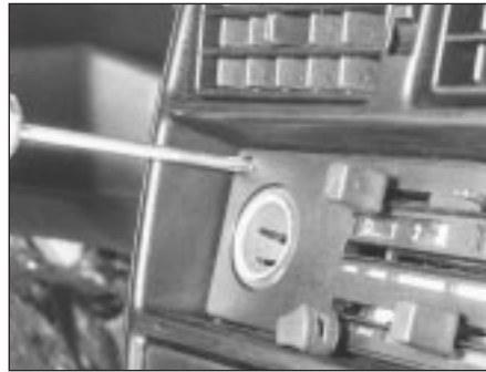
12.6A Heater control panel screw
