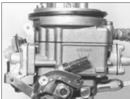
9B.2D Weber 32 TLF 4/250 carburettor from throttle linkage side
