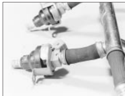
9C.81A Fuel injectors attached to fuel rail
