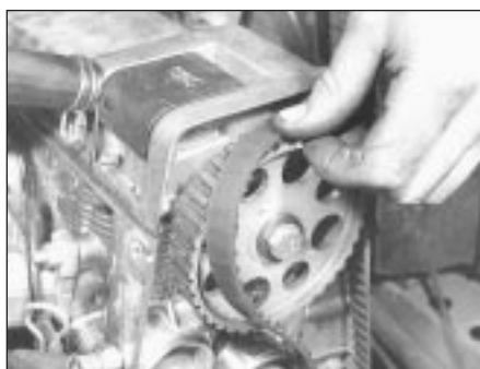
5B.12 Fitting the timing belt
