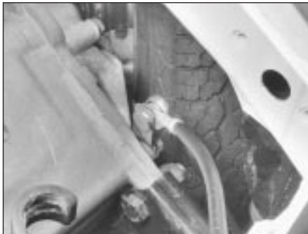
44.22B Transmission earth lead
