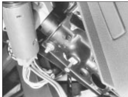
5.6 Steering column upper mounting
