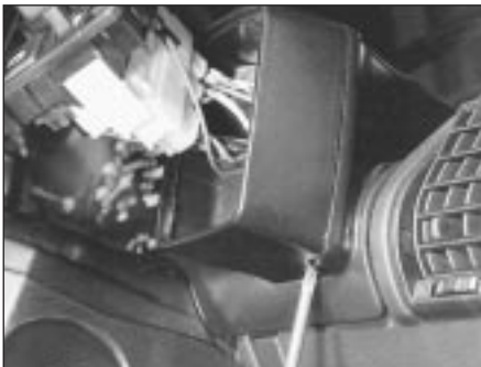
15.55A Facia switch housing lower screw removal on the 1301 cc Turbo ie model
