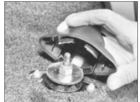
8.1 Rear shock absorber upper mounting cover
