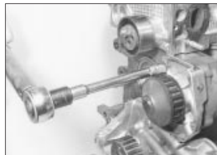
8A.17B Tightening the coolant pump bolts
