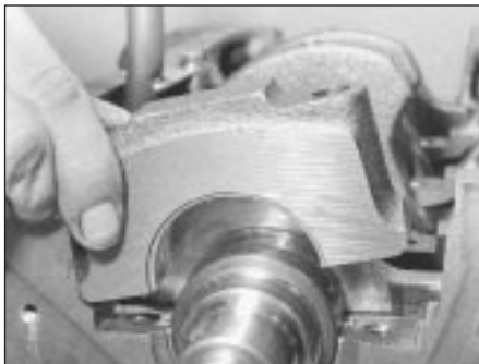
42.4A Number one main bearing cap
