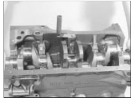
42.3 Lowering crankshaft into position
