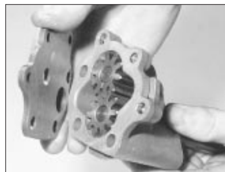
7B.179 Refitting the intermediate plate
