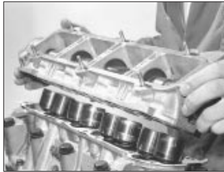
7B.84 Lowering the camshaft housing on to the cylinder head
