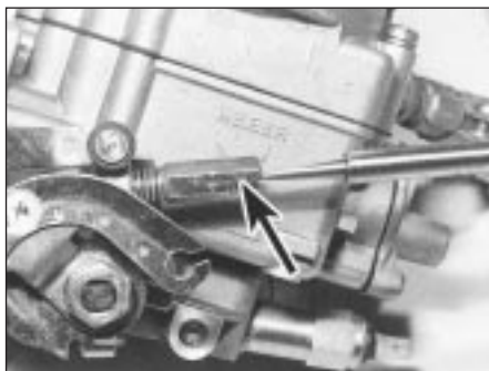
9B.6 Weber 32 TLF 4/250 carburettor idle speed screw (arrowed)
