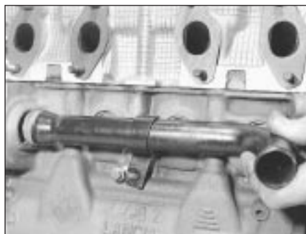
5D.30 Coolant distribution pipe
