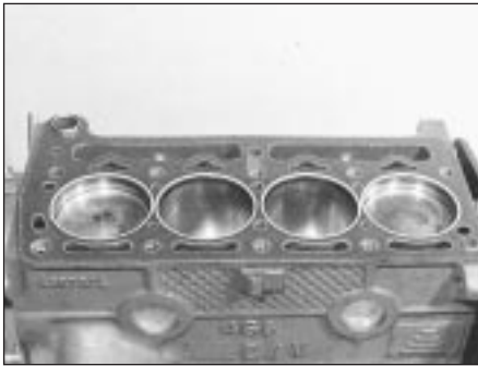
7.20 Cylinder head gasket
