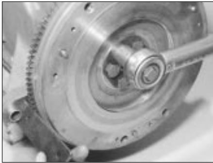
42.19 Tightening flywheel bolts
