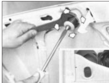
Fig. 12.2 Adjusting bonnet lock striker (Sec 8)
