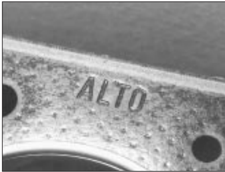
29.21A Cylinder head gasket top face marking
