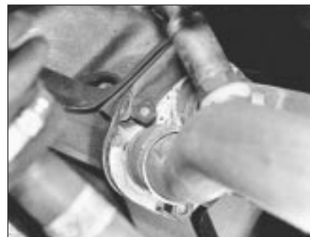
9D.71 Exhaust downpipe to manifold flange connection showing retaining nuts and locktabs
