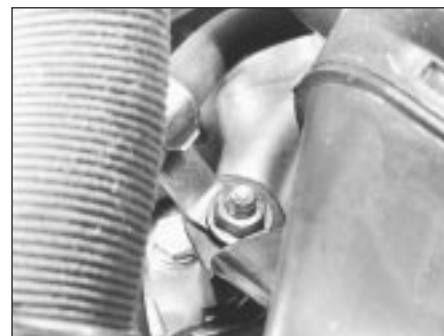
2.11B Air cleaner mounting bracket and pipe clip
