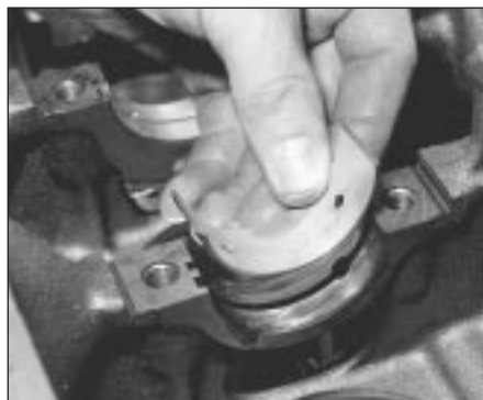
7D.6A No. 3 main bearing shell is plain . . .
