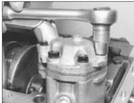
31.3 Bolting on the oil pump
