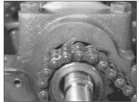
6.13C Self-tensioning links on inside of chain
