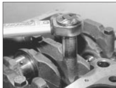
7DS.14 Tighten the main bearing cap bolts to the specified torque setting
