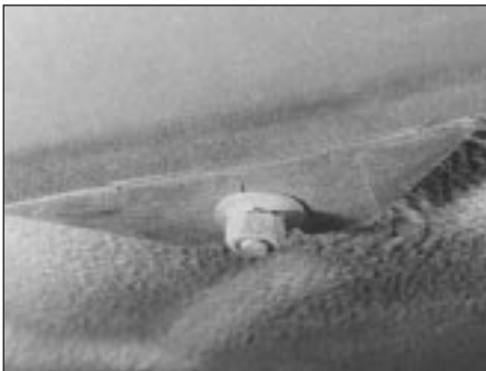
17.28 Rear bumper lower mounting nut
