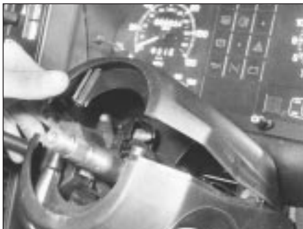
5.2 Removing steering column shrouds
