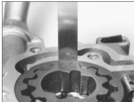
5B.74A Checking the oil pump gear-to-housing clearance
