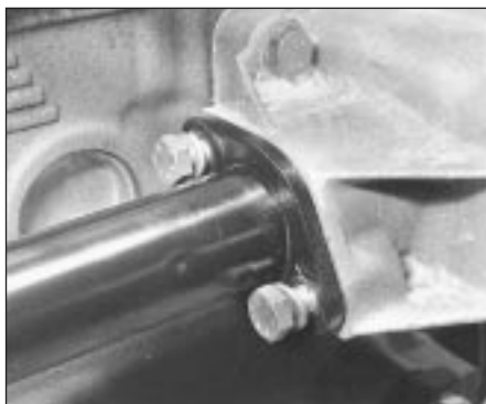
9.4 Coolant distribution tube at rear of pump
