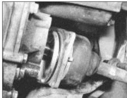
5C.25B Driveshaft joint gaiter withdrawn
