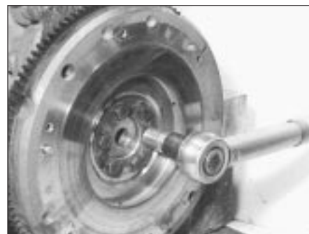
5D.14 Tightening a flywheel bolt
