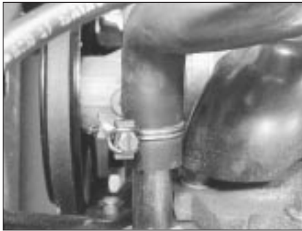
44.21A Heater hose at manifold
