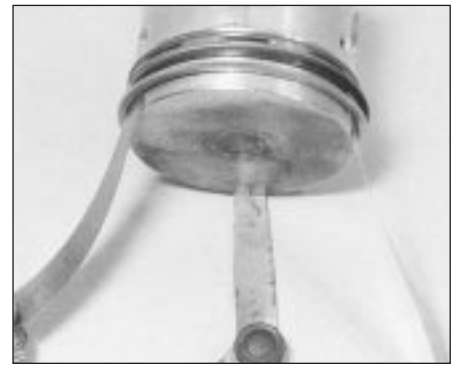
18.20 Using feeler blades to fit piston rings
