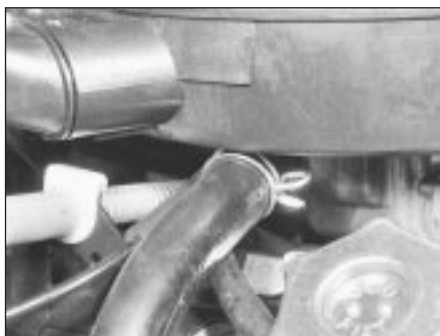
2.9 Crankcase vent hose at air cleaner
