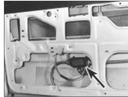
17.34C Door interior showing electric window motor (arrowed)
