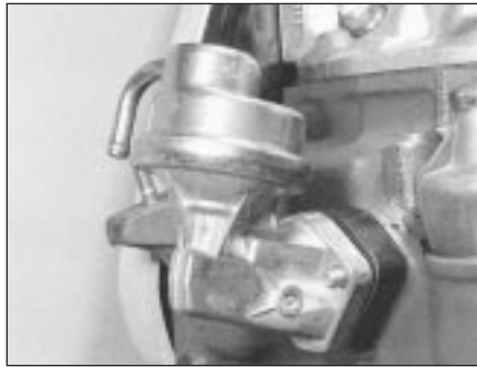
3.6A Fuel pump on mounting studs
