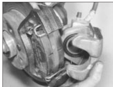
3.4 Removing the caliper unit
