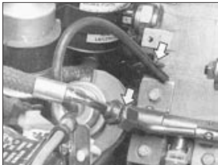
Fig. 13.60 Disconnecting the injector fuel supply pipe and fuel pressure regulator pipe on the 1372 cc Turbo ie engine (Sec 9E)
