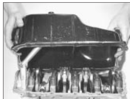
5C.60A Removing the sump pan
