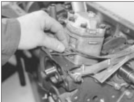
7B.166A Locate the new gasket . . .
