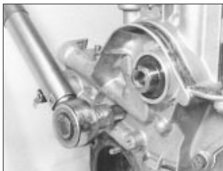
5D.12B Tightening an oil pump bolt
