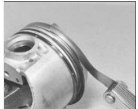
18.24A Checking piston ring groove clearance
