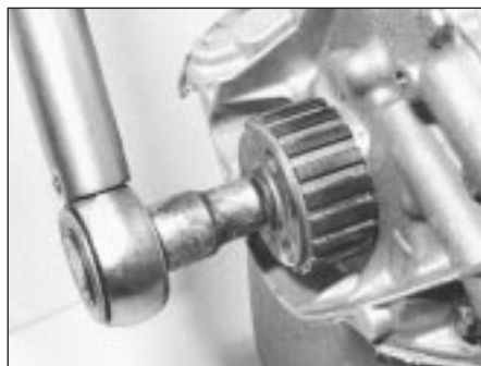
5D.16B Tightening the crankshaft sprocket bolt
