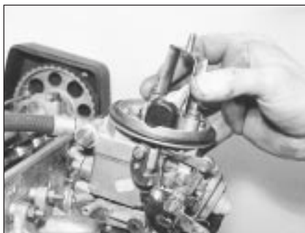
9B.18 Removing the Weber 32 TLF carburettor by gripping air cleaner mounting bracket
