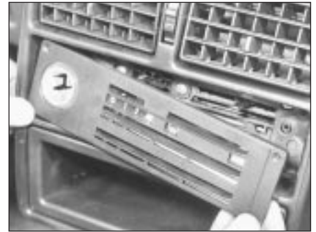
12.6B Removing heater control panel escutcheon
