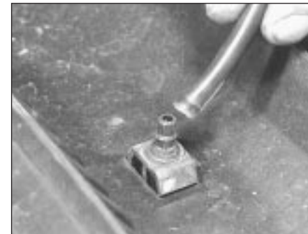
15.96B . . . and detach the windscreen washer hose
