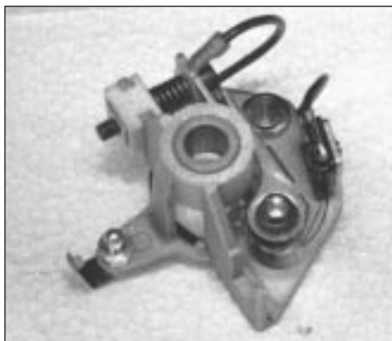
Fig. 4.3 Marelli contact breaker (Sec 2)
