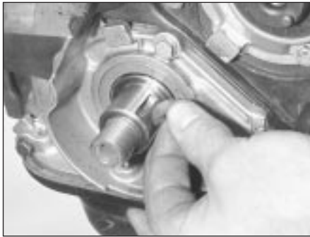
7B.43 Remove the crankshaft Woodruff key if it is loose
