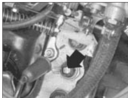
Fig. 1.9 Coolant temperature switch (Sec 13)
