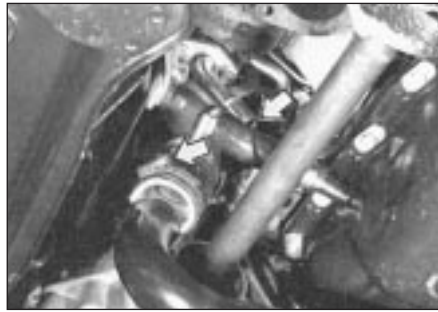
Fig. 13.67 Disconnect the heat exchanger air hose and the oil return pipe (turbocharger-to-sump) (Sec 9F)
