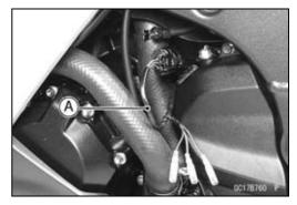
Connect a digital meter to the harness adapter leads.
