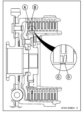
• Install the last friction plate [A] fitting the tangs in the grooves in the housing as shown.
