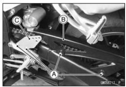
To adjust the spring preload, turn in the adjusting nut to the desired position and tighten the locknut using by hook wrenches [A] with the rear shock absorber attached the frame.
