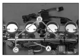
• Pull out the injectors [A] from the delivery pipe [B].
