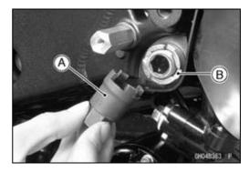
Using the Hexagon Wrench, turn the adjusting collar [A] counterclockwise to make the gap between the engine and adjusting collar.
