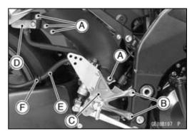
• Unscrew the mounting bolts [A], and detach the rear caliper [B] from the disc.
