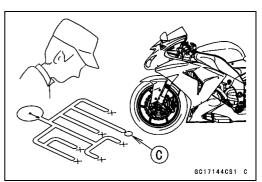
Even when the DFI system is operating normally, the warning indicator light (LED) and FI warning symbol may blink under strong electrical interference. Additional measures are not required. Turn the ignition switch OFF to stop the indicator light and symbol.
