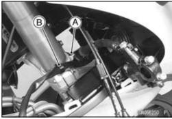
• Remove the left switch housing lead and ignition switch lead clamp [A].
