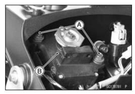
• Remove exhaust butterfly valve actuator pulley [A]. OHold the pulley with a suitable tool.
