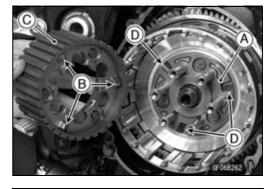
Install the four torque limiter springs [A] as shown.
