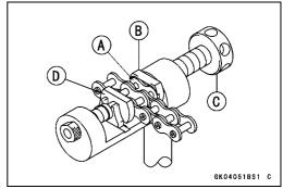
OInstall the handle lever [A] onto the pressure bolt (A) [B]. OTurn the handle lever, press in the link plate to the link pins.
