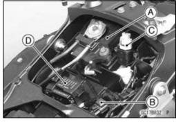
Inlet Air Temperature Sensor [A]
