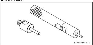
Valve Spring Compressor Adapter,  $\phi$ 24: 57001-1586
