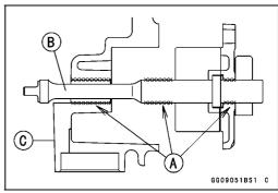
Install the following to the oil pump gear shaft [A].
