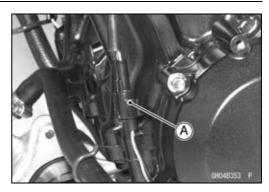
Remove: Gear Position Switch Lead Connector [A] Alternator Lead Connector [B]
