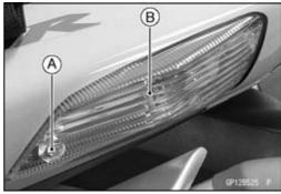
• Push and turn the rear turn signal light bulb [A] counterclockwise and remove it.
