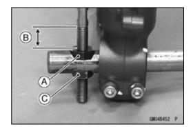
• Screw in one side nut [A] come out the piston rod nut.
