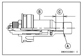
Set the fork spring compressor on the washer using the outer tube as a guide.
