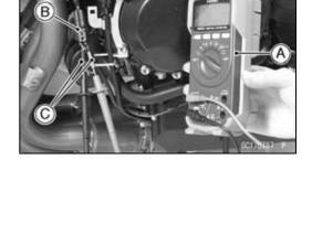
• Install the suitable plugs [A] on the fittings of the air suction valve covers [B], and shut off the secondary air.
