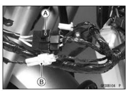
Put the current master key [A] at the antenna [B]. Insert the new user key 1 [C] to the new ignition switch [D] and turn it ON.
