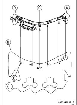
• Install the radiator in the projection [A] as shown.
