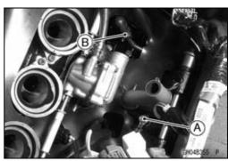
Support the engine with a suitable stand [A].
