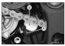
• Remove the pins [A] and springs from the shift drum.
