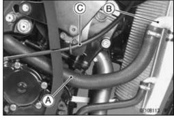
Remove Cap Bolt [A] Washer [B]
