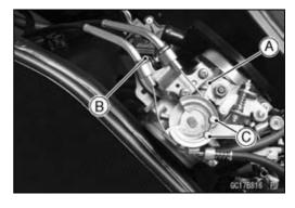
After removing the throttle body assy, stuff pieces of lint -free, clean cloths into the throttle body assy holders.
