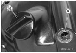
• Remove the needle bearings [A].
