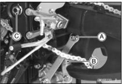
• Loosen the swingarm pivot collar locknut [A] using the nut wrench [B].
