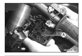
• Install the clutch lever [A] so that the mating surface [B] of the clutch lever clamps with punch mark [C] on the handlebar.
