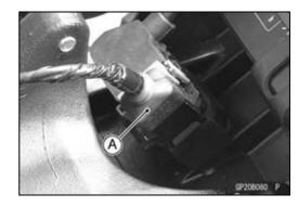
Pull out the main fuse [A] from the starter relay with needle nose pliers.
