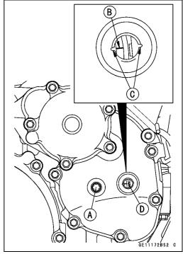
• Using a thickness gauge [A], measure the valve clearance between the cam and the valve lifter.
