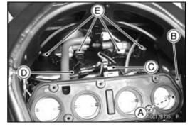
Water Temperature Sensor [A] Fuel Injectors #1, #2, #3, #4 [B]
