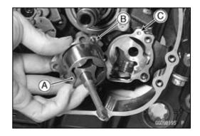
OTurn the oil pump gear shaft [A] so that the projection [B] in its shaft fits onto the slot [C] of the impeller shaft.
