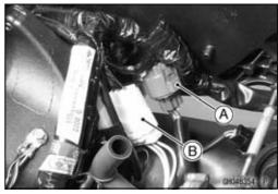
Remove: Engine Ground Cable Terminal Bolt [A] Starter Motor Cable [B]
