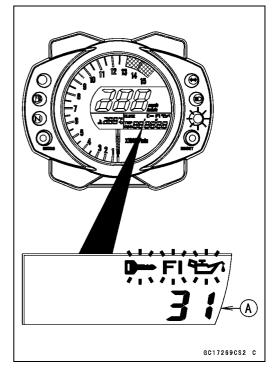
When the service code [A] is displayed, for first ask the rider about the conditions [B] of trouble, and then start to determine the cause of problem.
