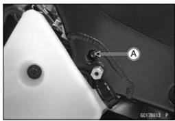
• Remove the throttle case [A] to make a throttle cable slack.
