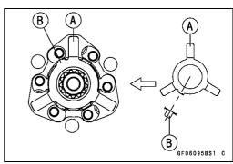
• Replace the clutch hub nut [A] with a new one.
