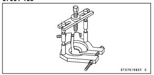
**Head Pipe Outer Race Press Shaft:** 57001-1075
