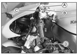
Oxygen Sensor #1 [A] (Europe Models) Oxygen Sensor #2 [B] (Europe Models)
