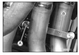
Remove: Radiator Fan Mounting Bolts [A] Radiator Fan [B]
