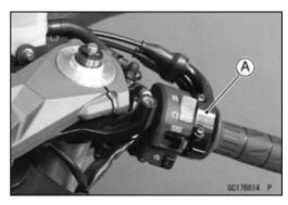
• Remove the adjuster screw [A] from the clamp [B].
