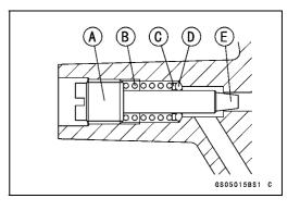
• Back out the same number of turns counted when first turned in. This is to set the screw to its original position.
