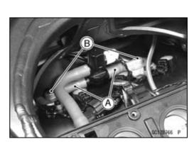
• Install the suitable plugs [A] on the fitting of the air suction valve covers [B], and shut off the secondary air.
