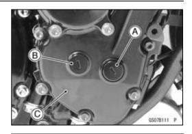
Using a wrench on the starter clutch bolt [A], turn the crankshaft clockwise until the line [B] (TDC mark for #1,4 pistons) on the starter clutch is aligned with the notch [C] in the edge of the timing inspection hole [D] in the crankshaft sensor cover.
