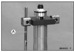
• Insert the lower end of the compression shaft [A] into the hole [B] of the holder bar.
