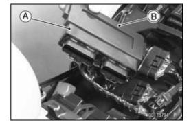
• Insert the slits of the rubber protector to the projections [A] of the rear fender front.
