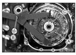
OUse the clutch holder with sharpened hook nose by grinding.
