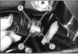
• Tighten the tensioner mounting bolts [A].
