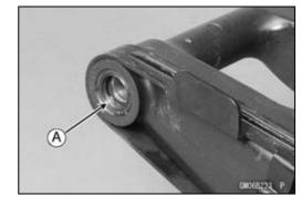
• Place the adjusting collar [A] into the frame [B] as shown.
