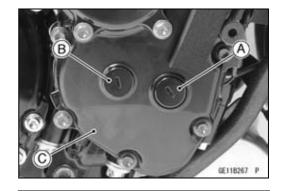
Using a wrench on the starter clutch bolt [A], turn the crankshaft clockwise until the line [B] (TDC mark for #1,4 pistons) on the starter clutch is aligned with the notch [C] in the edge of the timing inspection hole [D] in the starter clutch cover.
