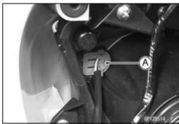
• Pull the bulb [A] out of the socket [B].
