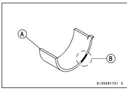
Install the new inserts in the connecting rod and check insert/crankpin clearance with the plastigage.
