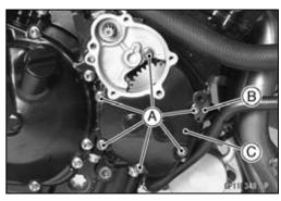
• Pull out the idle gear (starter clutch side) [A] with the shaft [B].
