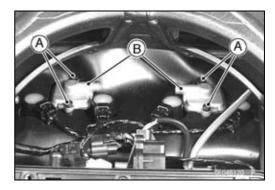
• Remove the air suction valves [A].
