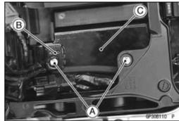
• Take out the ECU [A] and disconnect the connectors [B].
