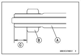
Check the distance [C] between the bottom end [A] of the top plug and rebound damping adjuster [B] with a pair of vernier caliper.
