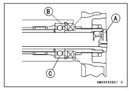
• Tighten the adjusting collar locknut [A] with the swingarm pivot nut wrench [B].
