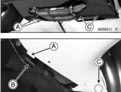
• Set the quick rivet [A] and push the core [B].
