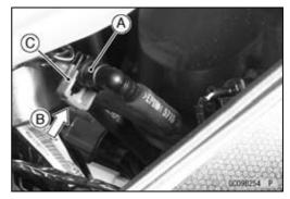
Push and pull [A] the hose joint [B] back and forth more than two times and make sure it is locked and doesn't come off.
