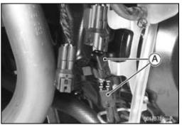
• Set the hand tester [A] to the  $\times$  1  $\Omega$  range and connect it to the terminals in each oxygen sensor lead connectors [B].
