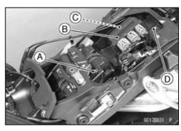
Exhaust Butterfly Valve Actuator [A]
