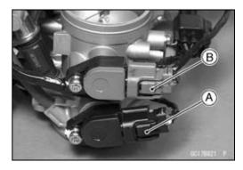
Disconnect: Subthrottle Valve Actuator Lead Connector [A] Inlet Air Pressure Sensor Connector [B]
