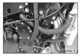
Speed Sensor [A] Gear Position Switch [B]
