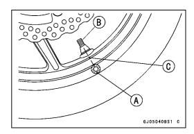
Lubricate the tire beads and rim flanges on both sides with a soap and water solution or rubber lubricant. This helps the tire beads slip off the rim flanges.
