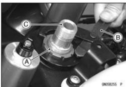
To remove the bearing outer races [A] pressed into the head pipe [B], insert a bar [C] into the recesses [D] of head pipe, and applying it to both recess alternately hammer it to drive the race out.
