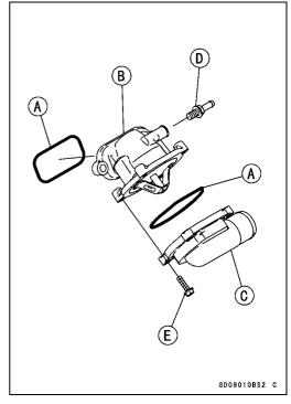
Install the thermostat housing.
