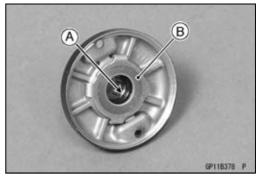
Align the marks [A] to assembly the yoke and the end covers.
