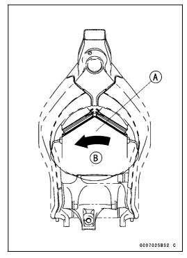
• Pull off the air ducts [A] from the frame.
