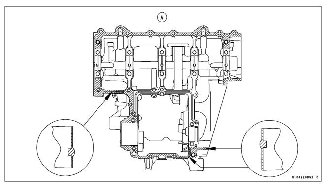
• Fit the lower crankcase half to the upper crankcase half.
