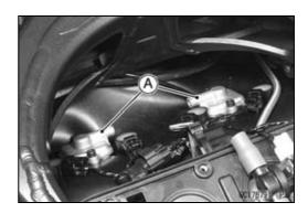
Measure the output voltage of the sensor with the connector joined.
