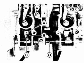
A. Choke Valve B. Choke Arm
