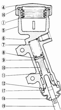
**NOTE:** The cups and spring are part of the piston assembly. Replace the piston assembly if any one of the cups or the spring requires replacement.
