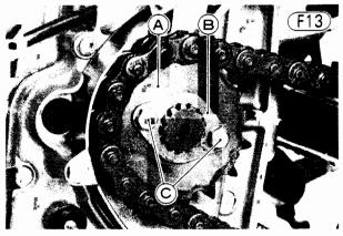
A. Engine Sprocket B. Holding Plate
