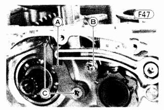
A. Bearing Stop B. Oil Pump Bolt
