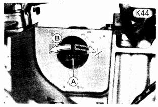
A. Starter Motor Idle Gear
