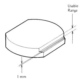
For the rear disc brake, if either pad is worn down through the stepped portion, replace both pads as a set.
