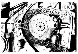
A. Engine Sprocket Holding Plate
