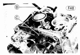
A. Gear Pusher (57001-319) B. Secondary Shaft Gear
