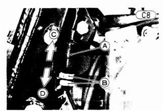
A. Brake Light Switch B. Mounting Nuts
