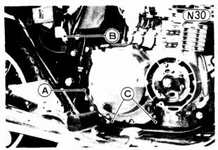
A. Pick-up Coil Lead B. 4-pin Connector
