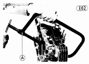
A. Valve Spring Compressor Assembly (57001-241)
