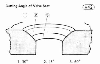
Next, use the  $30^{\circ}$  cutter (inlet valve seat only) to cut the surface inside the seating surface, and then use the  $60^{\circ}$  cutter to cut the outermost surface. Cut these two surfaces so that the seating surface will have the specified width.
