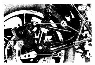
A. Torque Link Nuts B. Rear Axle
