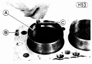
A. Piston Ring B. Cylinder Block
