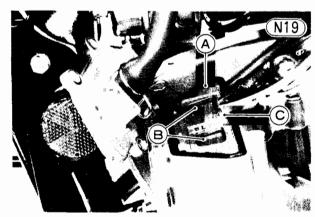
A. Valve Assembly B. Valve Reeds
