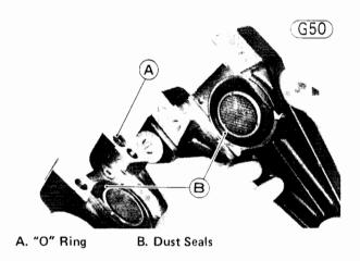
•Wrap each caliper half with a clean, heavy cloth, and remove each piston 6 by lightly applying compressed air to the brake fluid passage.
