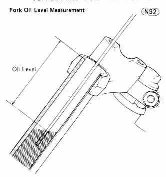
The operation of air front forks is especially dependent upon correct oil level. Higher level than specified may cause oil leakage and seal breakage. So be sure to maintain the specified level.
