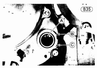
A. Engine Oil Level Gauge B. Upper Level Line
