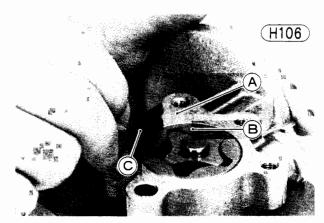
A. Pump Body B. Outer Rotor
