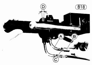
A. Accelerator Cable Elbow B. Adjusting Nut
