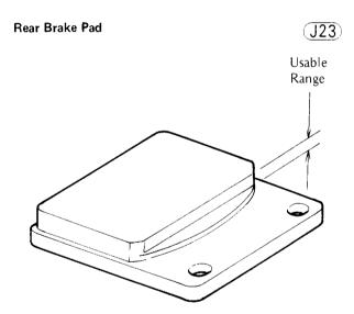
If any grease or oil spills on the pads, wash it off with trichloroethylene or a high flash-point solvent. Do not use one which will leave an oily residue. If the oil cannot be thoroughly clean off, replace the pads.
