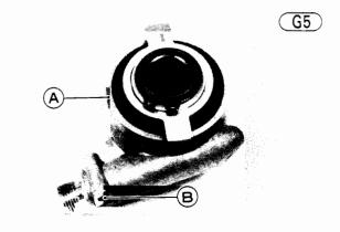
A. Speedometer Gear Housing
