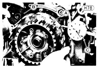
A. Clutch Housing Gear B. Secondary Shaft Gear
