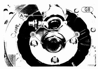
A. Speedometer Gear Housing
