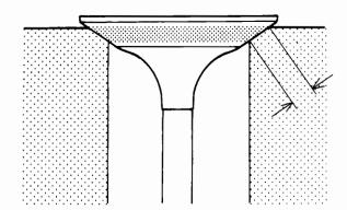
Valve/Valve Seat Contact Area
