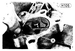
A. Outer Rotor B. Inner Rotor
