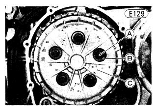
A. Clutch Spring Bolt B. Washer
