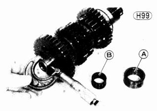
A. Needle Bearing Outer Race
