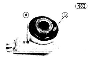
A. Speedometer Gear Housing
