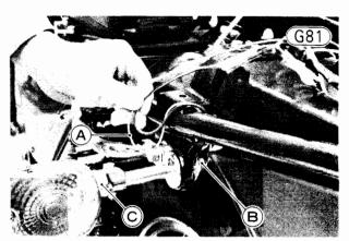
A. Turn Signal Lead **B.** Mounting Nut
