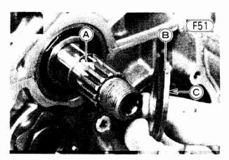
A. Drive Shaft B. Clutch Housing Spacer
