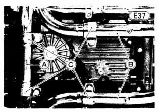
A. Connecting Pipe B. Exhaust Pipes
