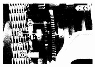
A. Idle Gear B. Circlip
