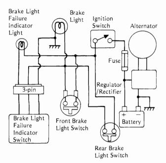
The front brake light switch, mounted on the front brake lever holder, is actuated when pressed by the front brake lever. The front brake light switch never requires adjustment, and so is not designed to be adjusted. It cannot be disassembled for repair and must be replaced when defective.
