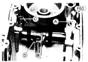
A. Positioning Bolt B. Shift Fork Guide Pin
