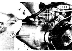
A. Starter Motor B. Terminal Nut
