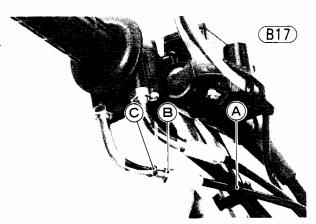
A. Decelerator Cable B. Adjusting Nut
