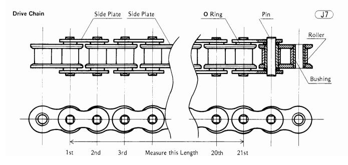
reduced by providing O rings  $\overline{to}$  seal in the lubricant between the pin and bushing. The wear between bushing and roller can be minimized by frequent and sufficient lubrication.
