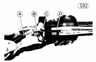
A. Clutch Cable B. Adjuster
