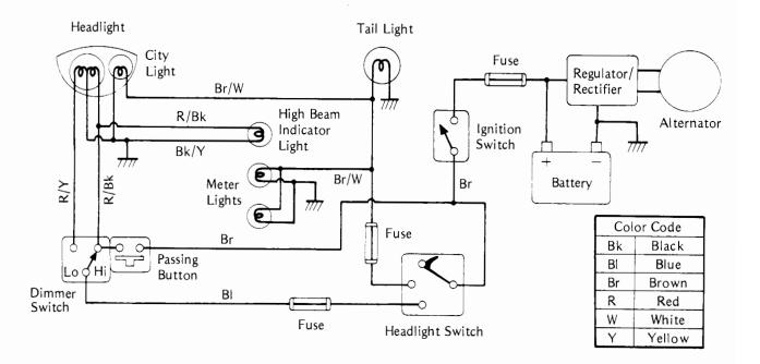
There is also a passing and horn button. This button is spring loaded and when the button is pushed to pass, the high beam light (but not the tail light) comes on as a passing signal to the driver of the vehicle ahead. The passing button will light the high beam light regardless of the headlight switch position, and the button will spring back and turn the light off as soon as it is released.
