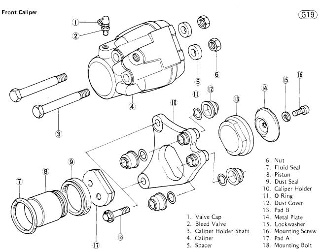
• Taking care not to damage the cylinder surface, remove the fluid seal 7 with a hook.
