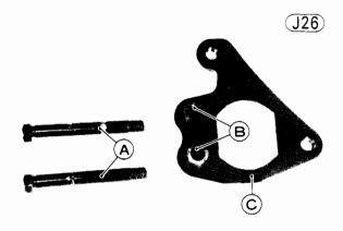
A. Caliper Holder Shafts B. "O" Rings
