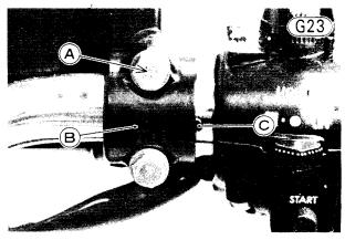
A. Tighten the upper clamp bolt first.
