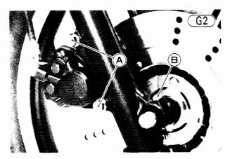
A. Caliper Mounting Bolts
