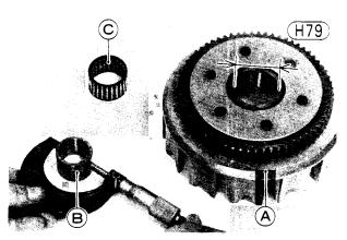
A. Clutch Housing B. Drive Shaft Sleeve
