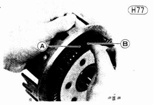
A. Clutch Housing Gear
